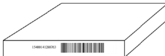
Figure 6b: Suggested Label Placement for Shallow Trays
